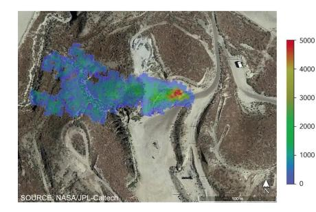
Methane plume detected by NASA identified a leaking gas line in California that the operator was able to repair
